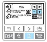
Press **–** to weaken the thread tension.
